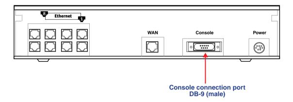
To connect the Netopia 4622 to your computer for serial console communication, use a console cable appropriate to your platform:
